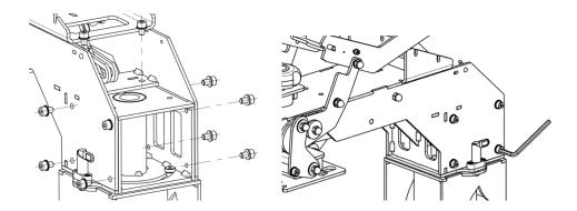
Remove the screws from the lever
