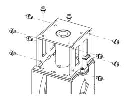
• Connect the heat press base with the heat press head.
