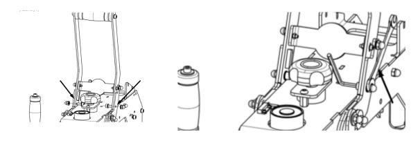
Connect the base plate with the heat press base (only the adapter is visible) and fix it in advance.
