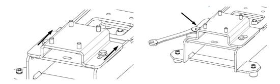
• Position the heat plate *HP7* in front of the connecting flange below the press lever on the *heat press base* at a slant and thread the 4 outer screws heads into the keyhole grooves on the flange plate.
