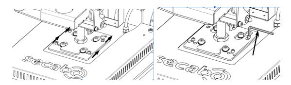
• Carefully tighten the screws with the supplied allen wrench. Attention, the heating plate can fall down as long as the screws are not tightened! Risk of injury!
